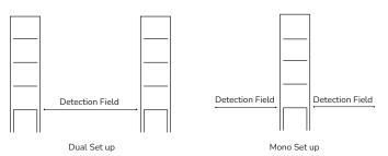
Detection ranges measured under low electrical noise conditions. Detection ranges under higher electrical noise conditions may decrease. For mono systems, total detection coverage (both sides of the antenna). For dual systems, detection coverage between the antennas.
