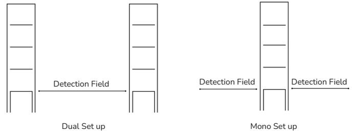
Detection ranges measured under low electrical noise conditions. Detection ranges under higher electrical noise conditions may decrease. For mono systems, total detection coverage (both sides of the antenna). For dual systems, detection coverage between the antennas.
